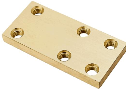
The Long D Plate (Part # 80329002) is made of brass and fastened to the back of a multi-cylinder MD Series Type D interlock to allow front mounting (see MD Series Data Sheet 1.4). The thickness of the Long D Plate is 3/8". To order this plate with your multi-cylinder MD Series Type D interlock, put the letter "P" in column fourteen of the interlock part number - reference the MD Series Ordering Guide.
