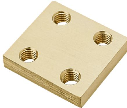
The Short D Plate (Part # 80329001) is made of brass and fastened to the back of a single cylinder MD Series Type D interlock to allow front mounting (see MD Series Data Sheet 1.4). The thickness of the Short D plate is 3/8". To order this plate with your MD Series Type D interlock, put the letter "P" in column fourteen of the interlock part number - reference the MD Series Ordering Guide.
