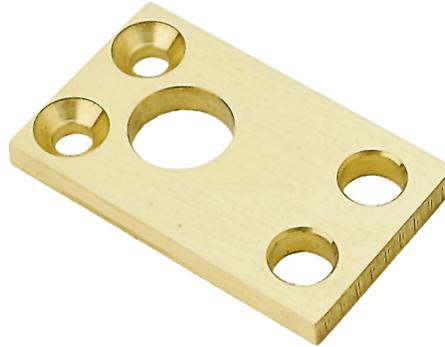
The FN Plate (Part # 155987001) is made of brass and fastened to the end of a MD Series Type FN interlock to allow alternative mounting scenarios (see MD Series Data Sheet 1.7). The thickness of the FN Plate is 1/4". To order this plate with your MD Series Type FN interlock, put the letter "P" in column fourteen of the interlock part number - reference the MD Series Ordering Guide. The plate (when ordered) will be bolted to your Type FN interlock.
